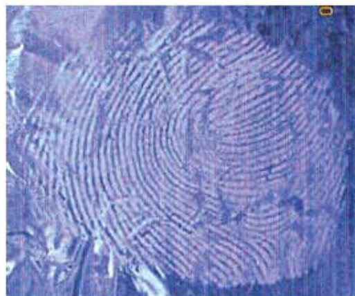
Fig. 7: Fingerprint developed by small particle reagent method on aluminium foil after it had remain suspended in water for 7 hours
